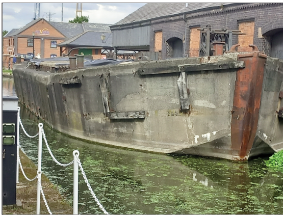
And this one is made of concrete...and floats!
